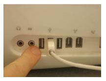
2) Plug the USB drive into the USB port
